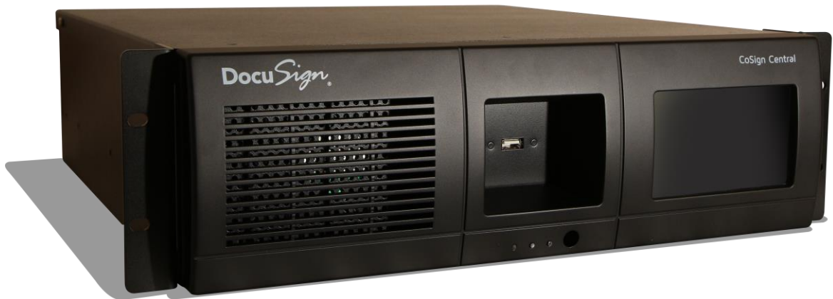
Figure 3 DocuSign Signature Appliance Central FIPS v8.0 Front Panel
