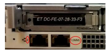
Figure 9 Ethernet connectors in DocuSign SA Enterprise Hardware version 8.0 Back Panel
